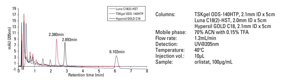
The TSKgel ODS-140HTP column yielded the shortest retention times in comparison to the other two competitive columns tested under identical chromatographic conditions.
