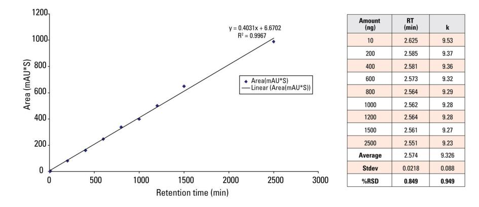
Peak area for orlistat was linear in the range of  $0.01 - 2.50\mu g$ . relative standard deviations for retention time and capacity factor were below 1% RSD in this range.
