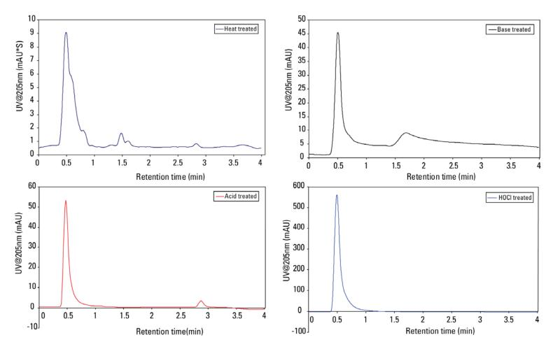
The orlistat peak disappeared upon forced degradation. This study shows that this column can be used for the forced degradation study of orlistat for quality control purposes.
